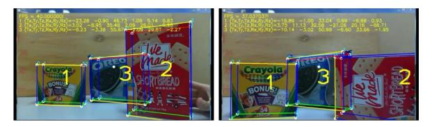
Figure 6. Experimental results of multi-object pose tracking of the proposed algorithm [32].
