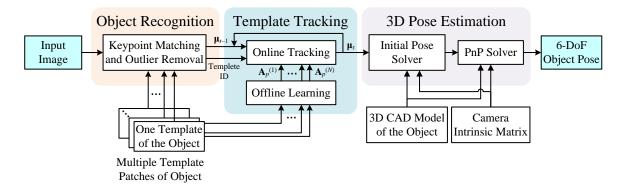
Figure 1. System framework of the proposed model-based object pose estimation algorithm.
