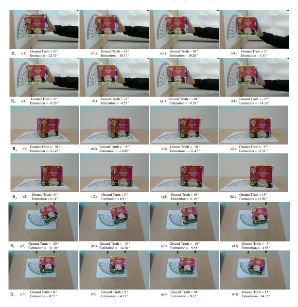
**Figure 5.** Experimental results of the proposed algorithm to estimate the rotation angles of the (**a1–h1**) *x*-axis, (**a2–h2**) *y*-axis and (**a3–h3**) *z*-axis of the OOI.
